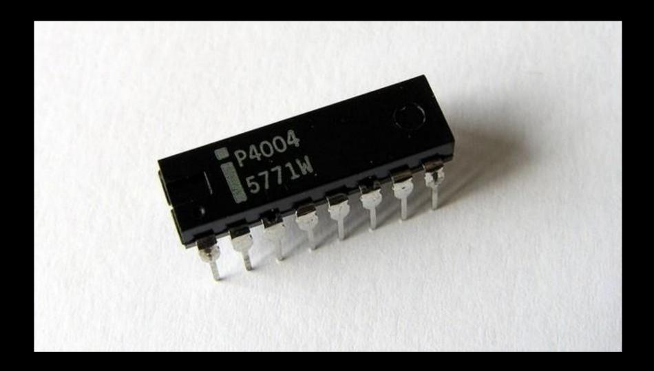
first commercial microprocessor chip - 2,300 transistors
